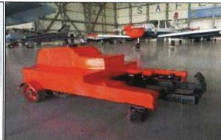
Gambar 6. *Prototype towing aircraft*
