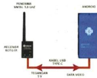
Gambar 2 Rangkaian Sistem *Receiver*
