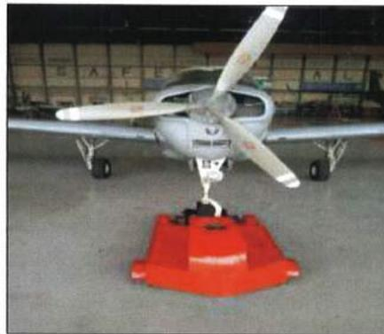
Gambar 5. Pengujian *prototype towing aircraft*
