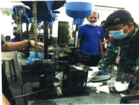
Gambar 4. Proses Cremping Amunisi caliber 20 mm
