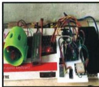
Gambar 2. Sistem pendorong USV
