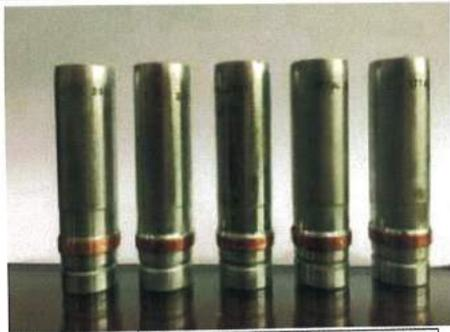
Gambar 2. Proyektil Kaliber 20 mm
