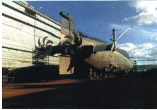
Gambar 1. High Skew Propeller
